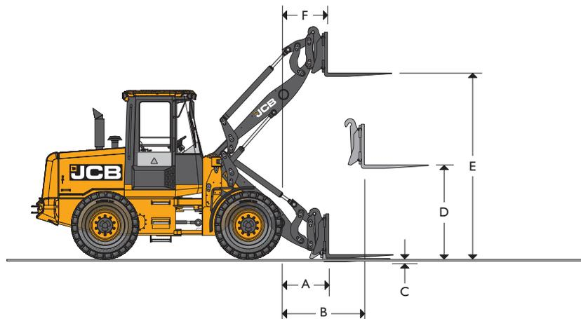
**HIGH LIFT LOADER DIMENSIONS – FORK FRAME WITH FORKS**
